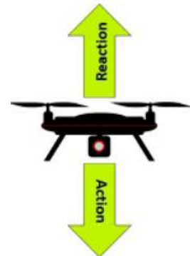
Figure 4 Upward motion of a quadcopter (Newton's third law)
