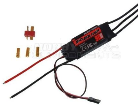
Figure 22: SKYWALKER 30A electronic speed controller
