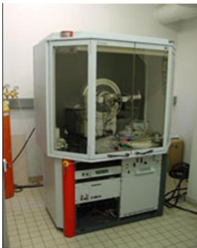
Figure III.3: Diffractomètre de type (BRUKER - AXS type D8 (LPTTSM Université de Constantine))
