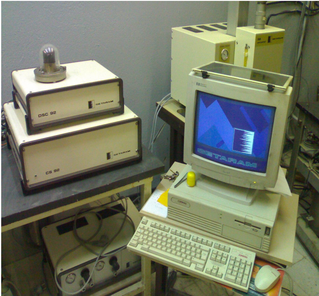
Figure III.5: DSC SETARAM 92 (LPTTSM Université de Constantine)
