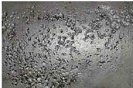
Figure. I. A. 3. Schematic representation of pitting corrosion [10].
