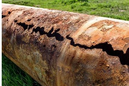
Figure. I. A. 7. Schematic representation of erosion corrosion [11].
