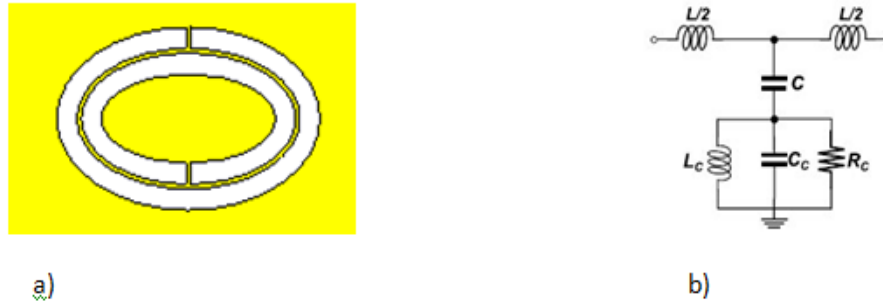
Fig. 2. (a) ECSRRs , (b) equivalent circuit model , with L and C for the unit length inductance and capacitance of the microstrip transmission line and ( RLC )c for DECSRRs.
