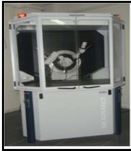
Fig.III.1 Image du diffractomètre BRUKER-AXS type D8
