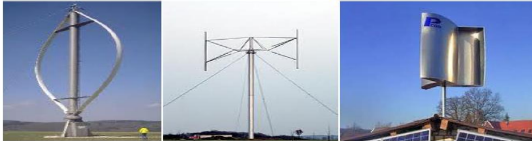
a) Classic Darrieus b) Turbines Darrieus turbines (H type) c) Savonius type turbine
