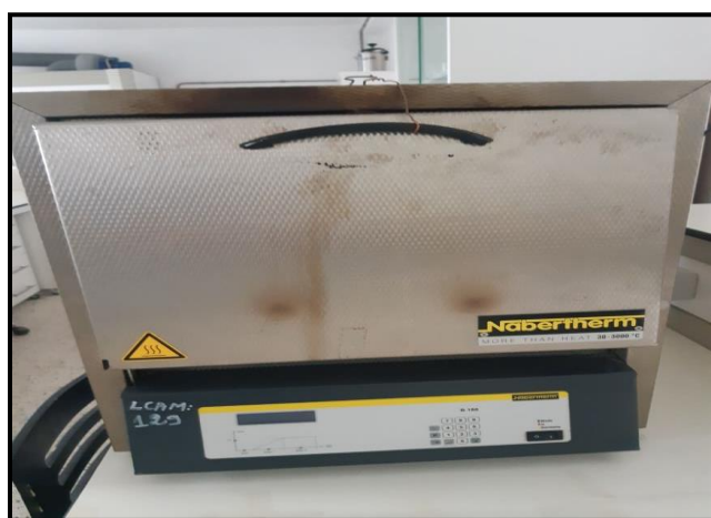
Figure IV.6: Four à moufle de type Nabertherm B-180 (30–3000 °C).
