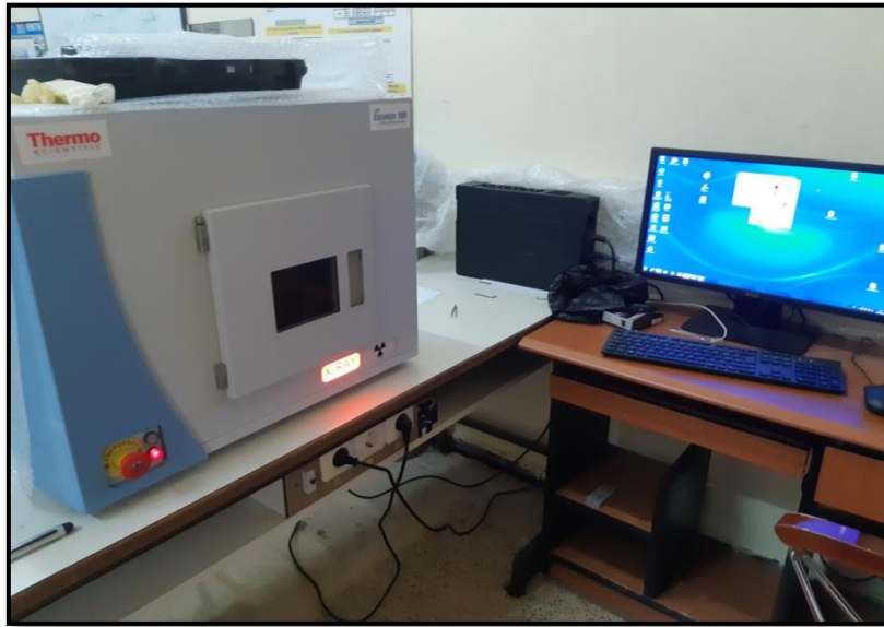
Figure II.12: Photographie du diffractomètre EQUINOX 100 (LMSSEF).
