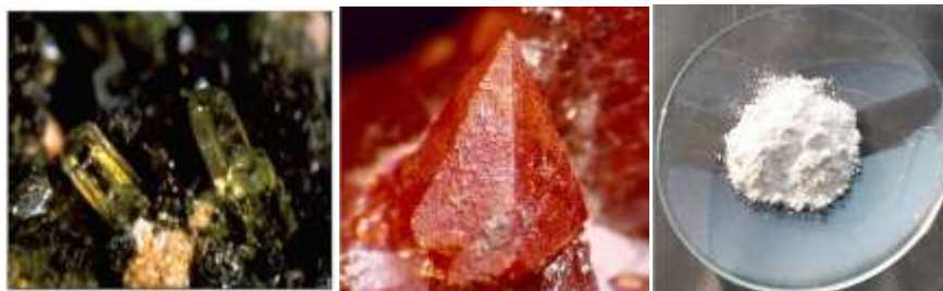
Figure I.2. Zinc oxide (ZnO) in a) natural form, b) crystal structures, c) amorphous powder [10].
