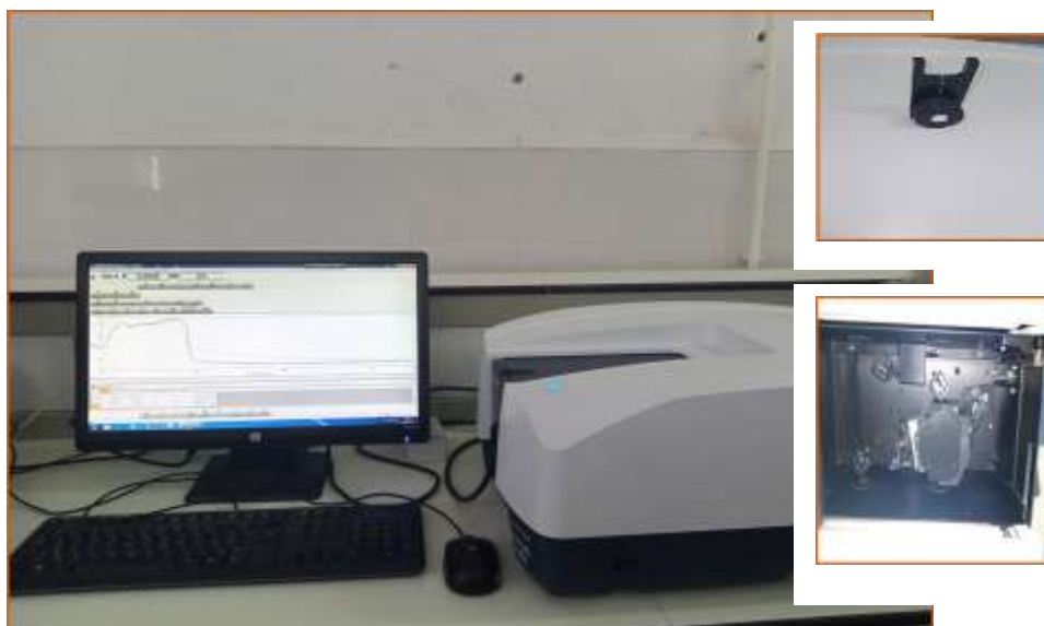
Figure II.8. Experimental device of the JaskoV-750 type UV-Vis spectrophotometer, measurement cell and powder cell.
