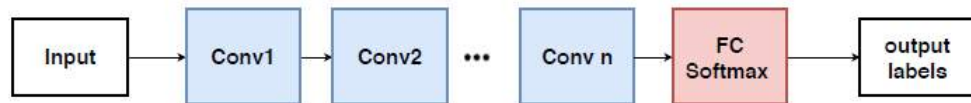
Figure 2.13: In fine-tuning process, all convolutional layers (blue layers) in the organization are fixed and slope is backpropagated through the completely associated (FC) layer as it were
