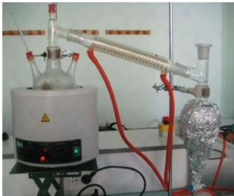
Figure 25: dispositif de l'hydro distillation
