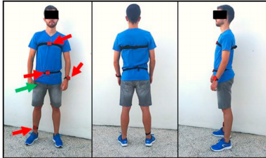
Figure 4.4: Location of the sensors (red arrows) and the smartphone (green arrow) on the subject for the UMAFall dataset (297)
