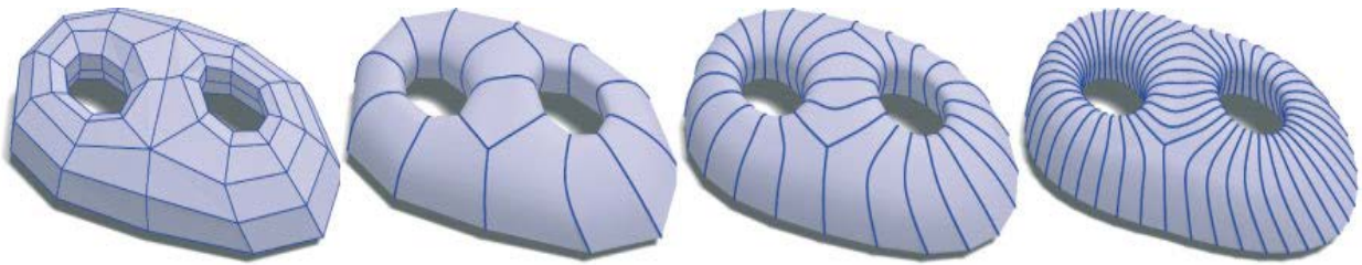
Figure 4-12: Ruled surfaces consisting of curves (Pottmann, 2010)
