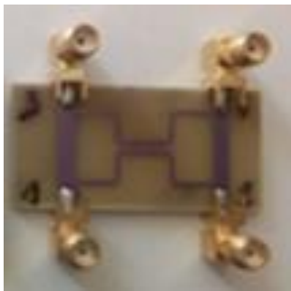
Figure 2. Three types of COD directional couplers with Input, through, isolation and coupled port.
