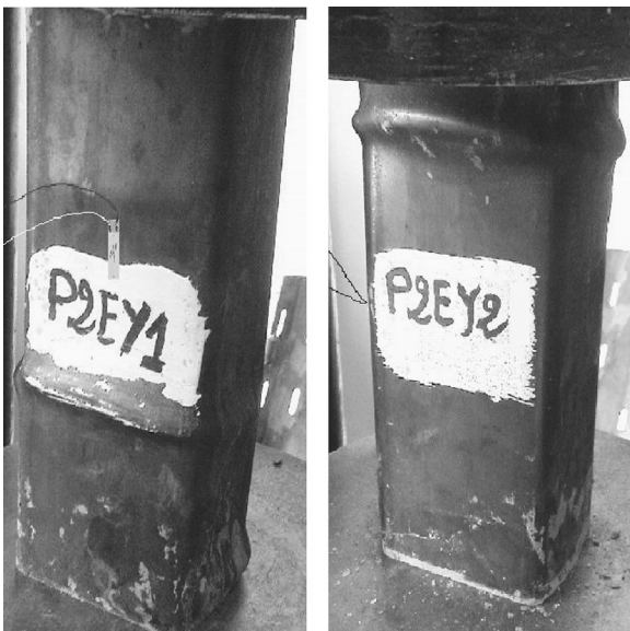
Fig. 12. P2EY1 and P2EY2 columns after test.
