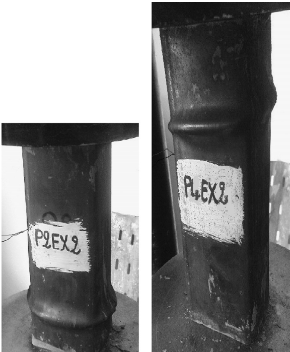
Fig. 11. P2EX2 and P4EX2 columns after test.
