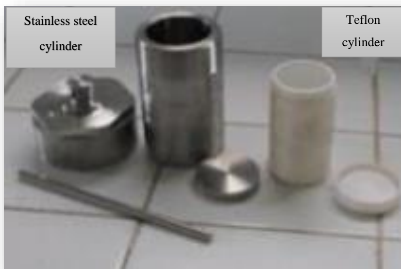
Fig.II.1 : General-purpose autoclave popularly used for hydrothermal synthesis.
