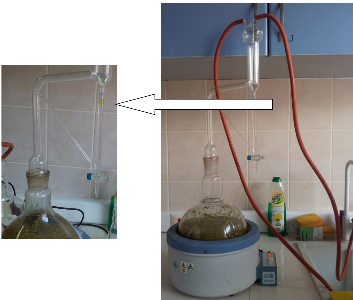
Figure 33. Clevenger apparatus for essential oil extraction
