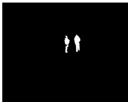
Fig.13. Localization or contour detection of two suspect persons by SVM method.
