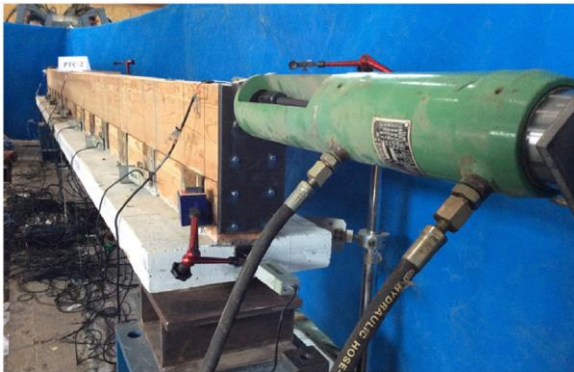
(a) Applying prestress using the tensile jack
