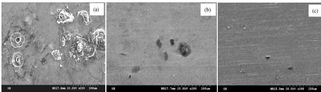
Fig. I.14. SEM surface morphology of (a) SS316L, (b) TiN, and (c) TiAlN coatings after corrosion tests in a 3.5wt.% NaCl solution [127].
