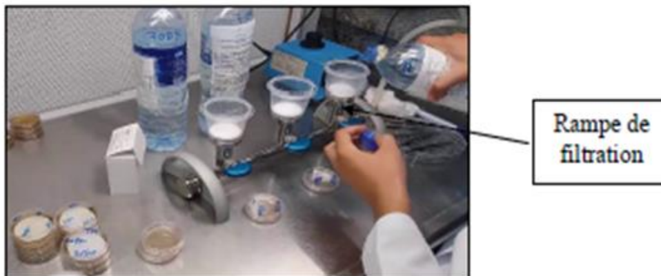
Figure 23: Rampe de filtration.
