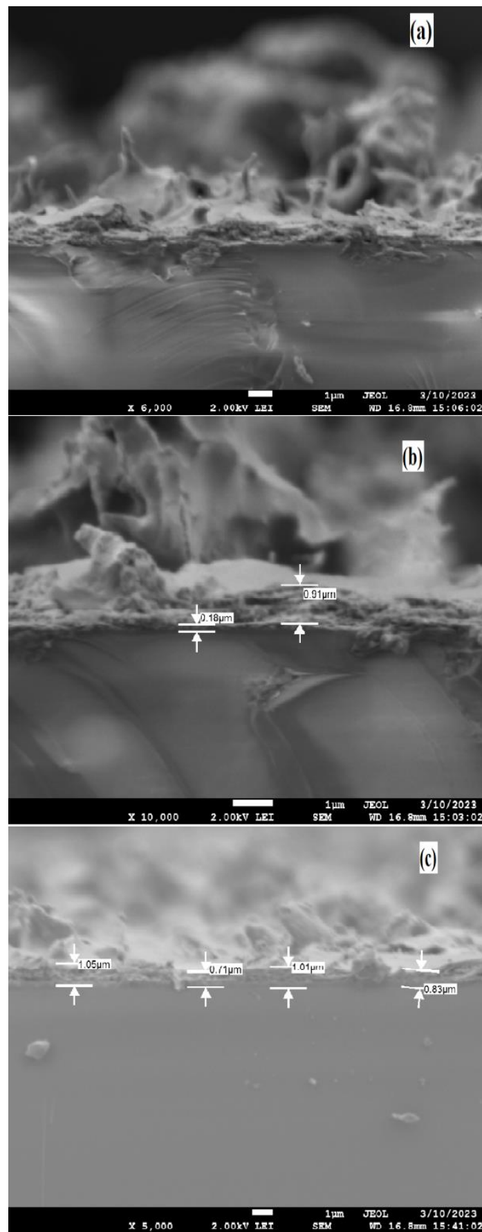
Figure 4.6: \text{Fe}_2\text{O}_3 thin films SEM images cross section morphology.
