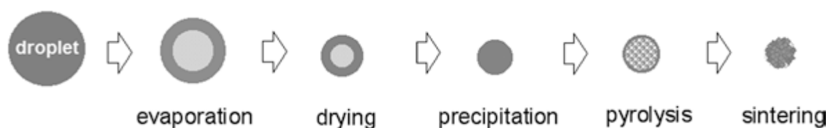
Figure 1.13: Steps of powder production during the spray-pyrolysis [79].
