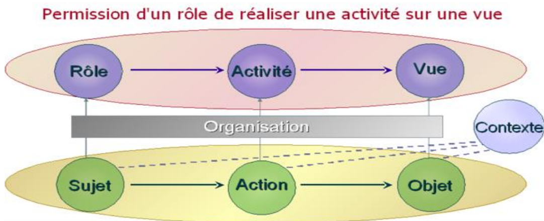
Figure. I. 4: Schéma montrant un modèle ORBAC (Organization Based Access Control).[18]
