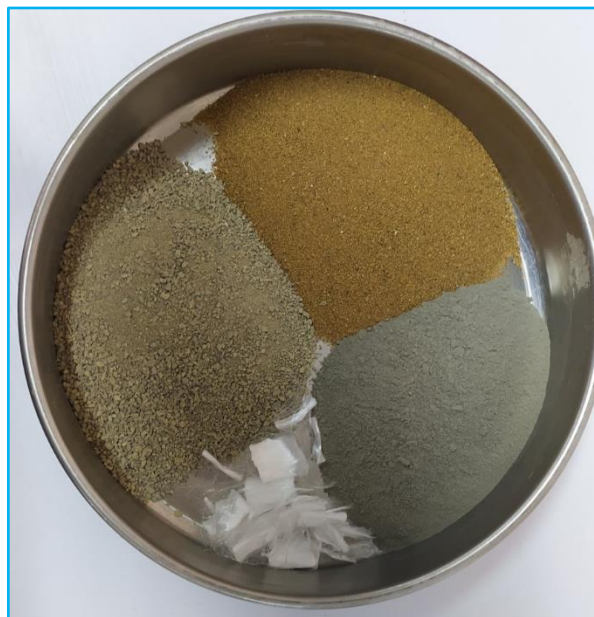
Figure 2.1 Sable, ciment, sol compressible et fibre PP.
