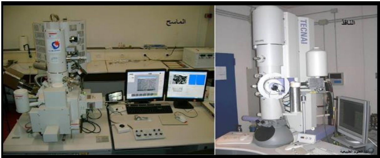
Figure 03: Images of transmission electron microscopes (right) and scanning electron microscopes (left).
