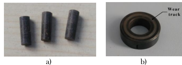
Figure 1. a) Cylindrical specimens and b) disc used in friction tests
