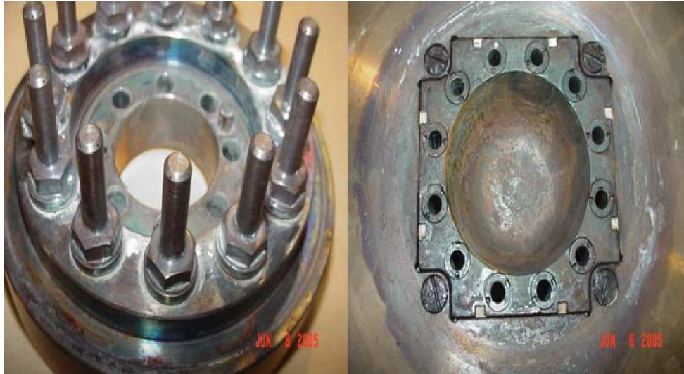
Fig.III.9: (a) Photograph of the fuel injectors and (b) Top view of the burner with the central cavity. [154]
