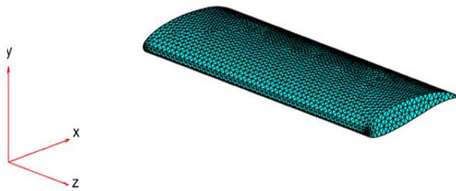
Figure 4.5: Finite element mesh of wing with tetrahedral elements.
